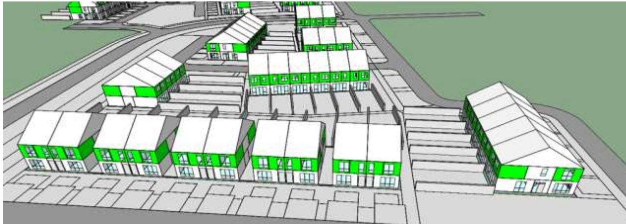
Above: Bedroom ADF results of Character Area 5 viewed from the South.
