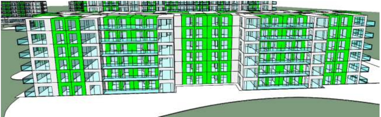
Above: Bedroom ADF results of the Block 1 from the east
