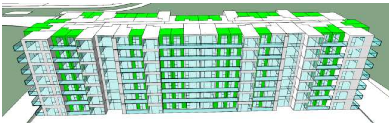
Above: Bedroom ADF results of the Block 2 from the east
