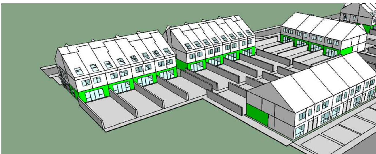
Above: Kitchen ADF results of Character Area 4 viewed from the Street.
