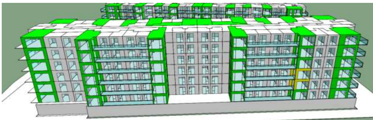
Above: Kitchen/Living ADF results of Apartment Block 2 viewed from the west
